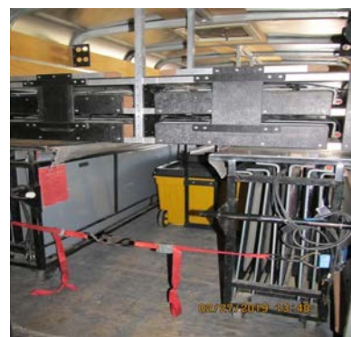
Figure 10 (Rear compartment: vertical stops installed across horizontal slots, yellow chest far in against black chest, red strap tight across touchpad caddies)
