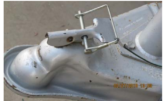
Figure 2 (Secured tongue latch with cotter pin in place)
