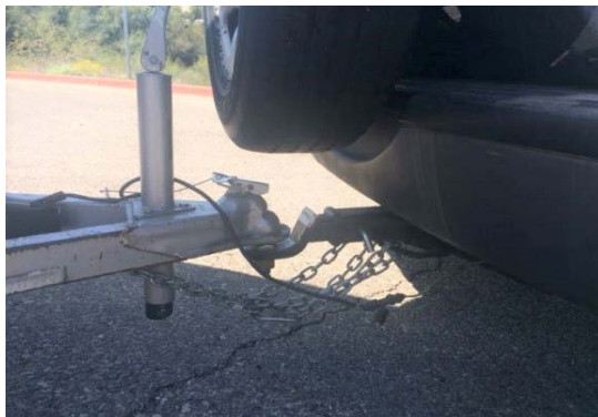
Figure 3 (Wheel removed from tongue jack; tongue jack pole retracted and trailer lighting harness cable above tongue)
