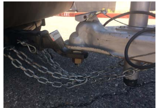
Figure 4 (Safety chains crossed under tongue and connected to hitch with reduced slack via hooks connected to links on chains)
