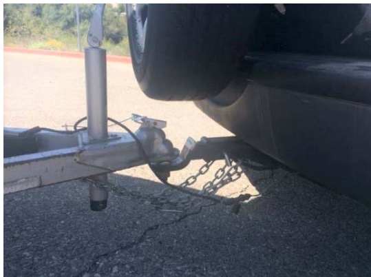
Figure 3 (Caster wheel removed from tongue jack; tongue jack pole fully retracted; trailer lighting harness cable above tongue and connected to vehicle)
