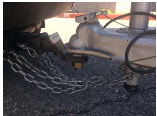
Figure 4 (Safety chains diagonally crossed under tongue and connected to hitch with reduced slack and even lengths via hooks connected to links on chains)
