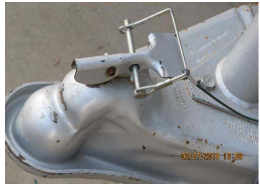
Figure 2 (Secured tongue latch with cotter pin in place)
